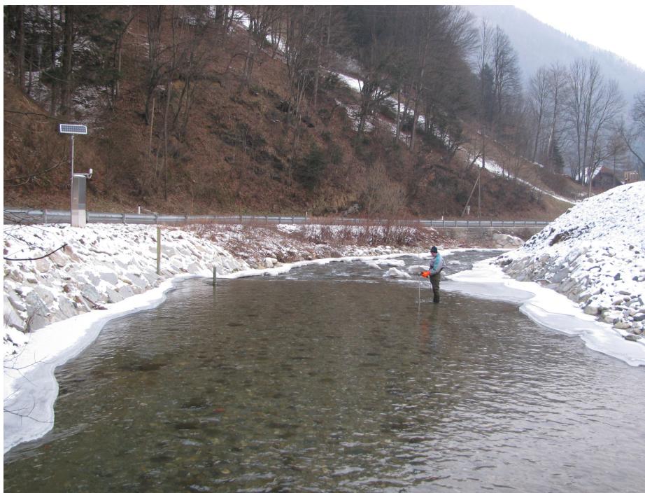
Meritev pretoka na Radoljni 7. januarja 2009 (foto: arhiv ARSO) Discharge measurement on the Radoljna stream on 7 January 2009 (Photo: Agency archives)
